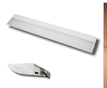
LED Linear Light for cove lighting Mounting method : wall mounted Material : extruded aluminium housing. PC Diffuser. ABS Cover. Standard finishes : aluminium IP Rating : IP44 Customized RAL upon request. Dimmable driver available upon request.
